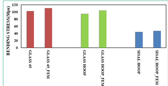
Figure 10: Bending strength comparison ( Experiment V/s FEA).
