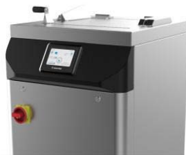
Figure 2: Shrinkage Testing Instrument DYNAWASH, James Heal, UK.
