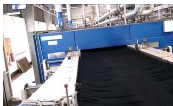
Figure 3: Heat Setting Conducting Stenter Machine (Heat Setting Going On).
