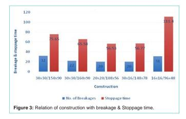
drop wire) and R (reed) zones. It was observed that more time was taken to repair a break in the D-H and H-R zones were due to the location of the break in an inconvenient place. Apart from this extra effort is required to reach, locate the heald wire and to pass the warp through it.
