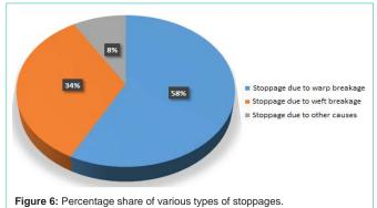
which was single end breakage and bunch breakage. The bunch breaks were the breakages where several warp threads were broken together. It was gathered that there are several reason for bunch breakages; some of the important reasons for bunch breakages were (i) the presence of lump which generated in the sizing section. Lump
