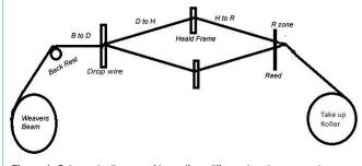
Figure 1: Schematic diagram of loom (four different breakage areas).
