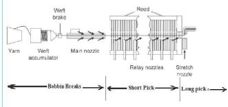
Figure 2: Zone wise weft breakage.
