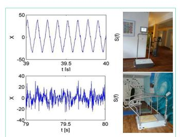
Figure 1: Left: Modes of vibration of two different modern devices for vibration training.
