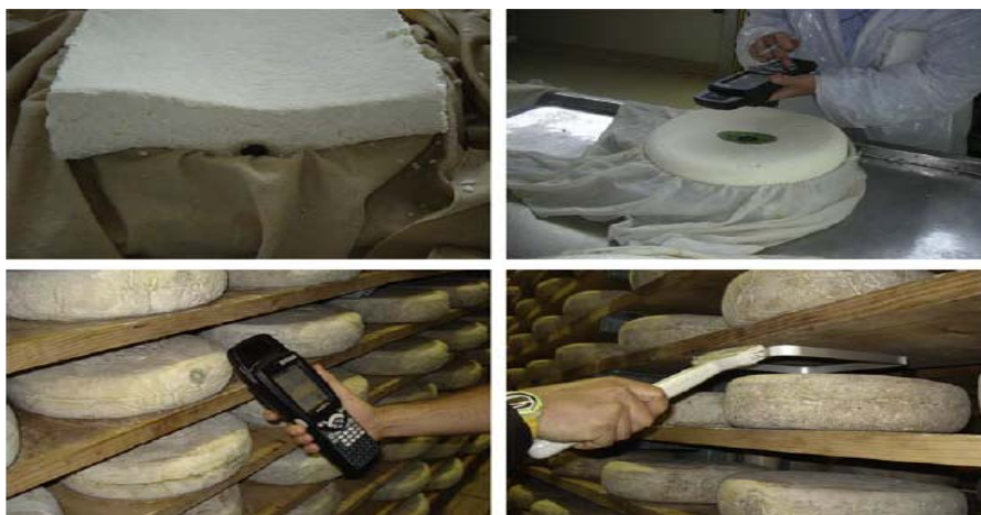
Figure 2: Cheese wheels identified by means of circular LF or HF tags. Transponders are applied under a casein disk during curd molding on the side (up, left), or on the cheese wheel face (up, right). During ripening the remains included in the cheese rind and can be detected by different handled models when placed on shelves in the storage room (down, left and right figures).
